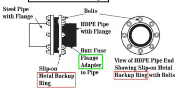
A backup ring is a metal ring used with bolts to make a secure connection to a pipe flange, a pump or valve.
